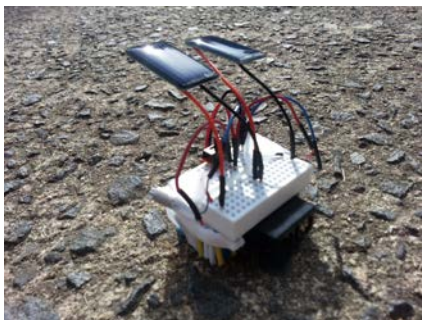
Figure 4: Solar powered Bristlebot
